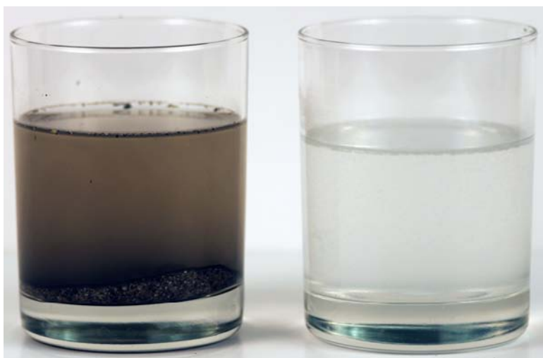
Left: Sand in a glass of water will settle to the bottom over time. Right: Salt mixed with water remains a solution.
