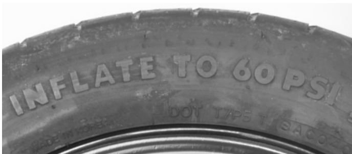
PSI is a measure of pounds per square inch, or air pressure.
